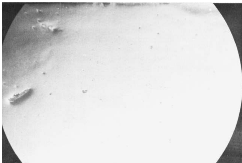
FIGURE 1 MBBA liquid crystal layer 30 \mu\text{m} thick with asymmetric anchoring: strong and weak realized with SiO under vacuum evaporation and soap rubbing respectively.
